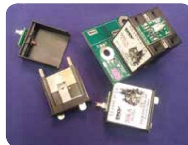
**Thermally Protected Metal Oxide Varistor (TpMOV) "Fail Safe Device"**
