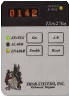
The standard monitoring package has solid state indicators for system status. This monitoring system provides two (2) individual LEDs for visual indication of Green (Power On) and Red (Service Required).
